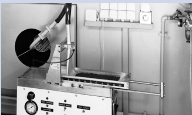
Figure 4: Dust feed device with ejector tube in front of mixer opening with perforated plate of test section.
