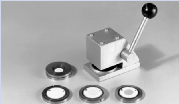
Figure 3: Target holder for filter papers used for opacity tests.
